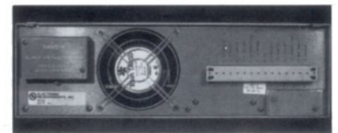
Rear View: Input, output, and programming terminals are covered for operator safety.
